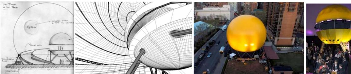
Entry into the structure began with a lightweight lattice portico which joined onto the tetrahedral frame and opened into a large 85 foot diameter dome shaped space where the exhibit began. The exhibit continued along a curved ramp which ascended a full floor until one reached a spherical geode which contained a small cinema. The cinema showed a 360 degree film about the new product.
