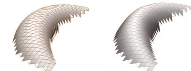
After locking in the shape, we began to look at the pillow cladding system which became much more efficient as a series of pneumatic strips rather than as defined diamond shapes, saving on inflation tubes, gasketing, etc.
