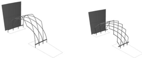
Next we examined the surface as both a pure toroid and as an inverted catenary hanging surface. Although the steel sizes were able to be reduced by 25%, the grid had become an element net made of straight components changing the design form considerably as shown below. We opted to stay with the rolled tubes, especially since they were all a single radius, saving rolling costs.
